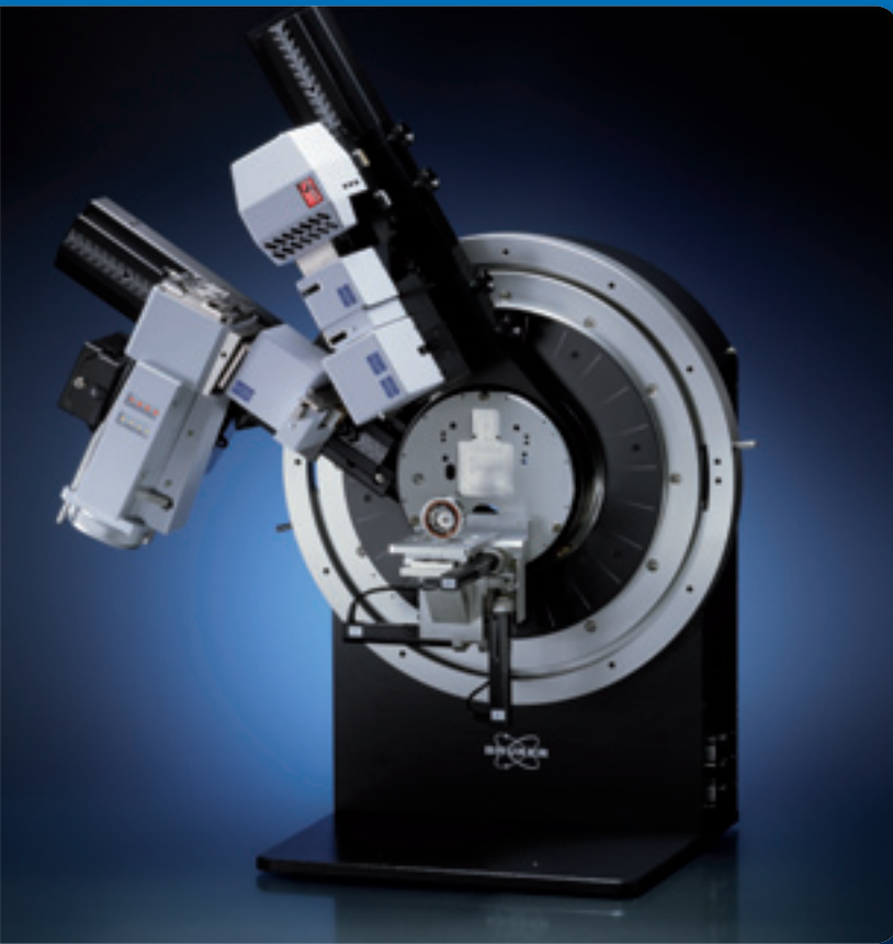
Stress measurements in iso-inclination (omega) mode
