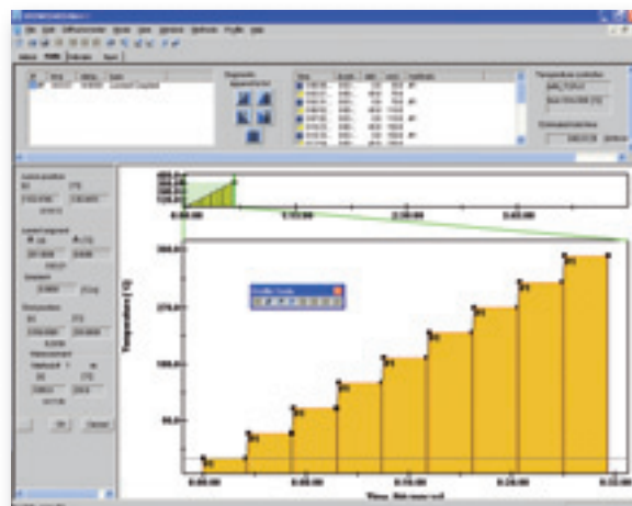
DIFFRAC.WIZARD to set up high-temperature experiments
