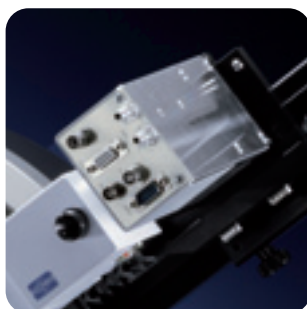
SOL-XE energy-dispersive detector
